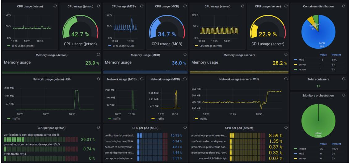
The entire architecture is monitored from a single web-based dashboard, accessible from any device
